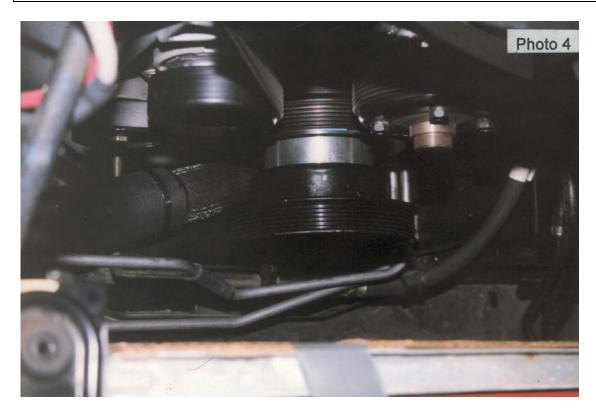
6. **Vortech Only** - Assemble and fit bracket as per drawing below. Remove power steering pulley, and fit counter-sunk bolts into bracket end. Fit bracket and check alignment.
