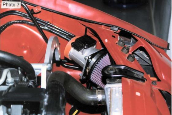
9. Fit supercharger to bracket with bolts supplied,  $5 \times 1 \frac{1}{4} \times \frac{3}{8}$ NC cap bolts. Fit idler pulley assembly to bracket, just nip it up. Check the position of the scroll.
