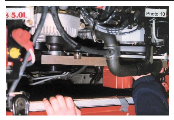
11. Fit the blower belt provided. Tension belt idler pulley only. Tension belt tightly enough to eliminate slippage. Re-tension the belt after 500km. Do not overtighten the belt.
