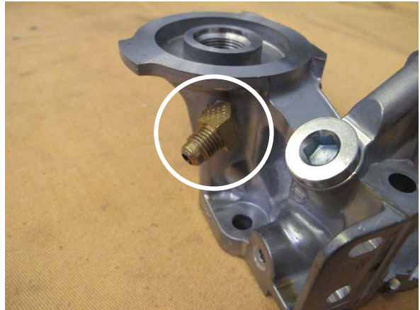
Fig. 1-p: Install 1/8" NPT 45° x -4 JIC Fitting
