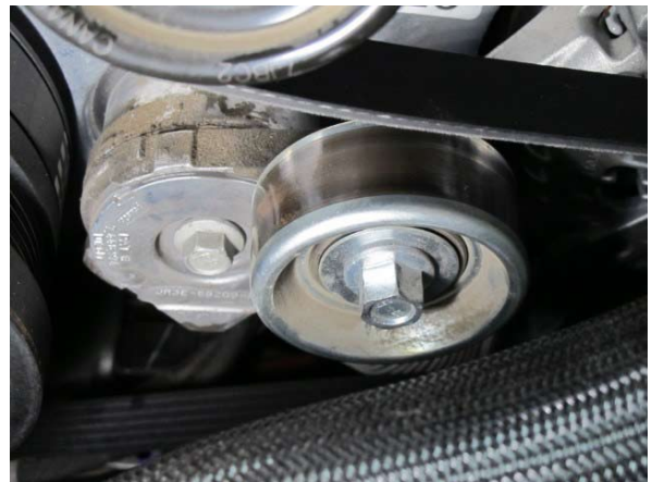
Fig. 1-b: Remove Belt Tensioner
