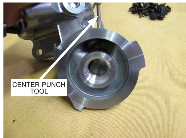
Fig. 1-l: Verify Center Punch Location
