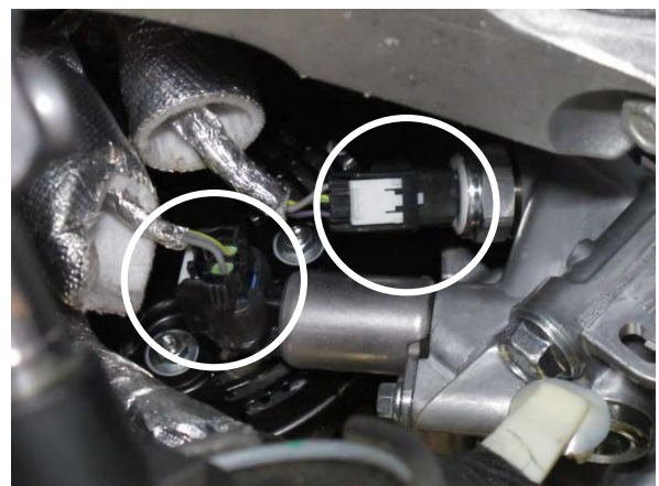
Fig. 1-i: Unplug Oil Sending Unit And Oil Control Solenoid
