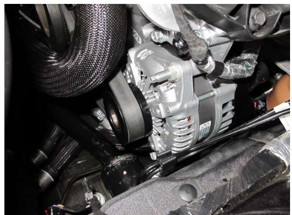
Fig. 1-c: Carefully Remove Alternator
