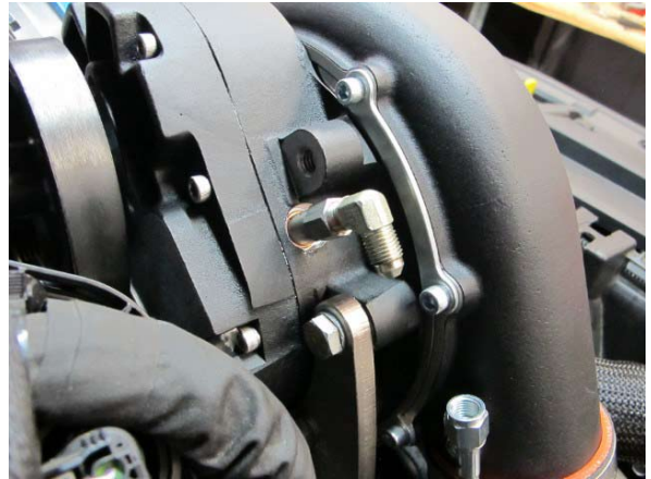
Fig. 1-v: Install 1/8" NPT 90° x -4 JIC Fitting
