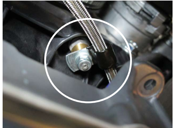
Fig. 1-s: Route Steel Braided Oil Feed Line Through Adel Clamp
