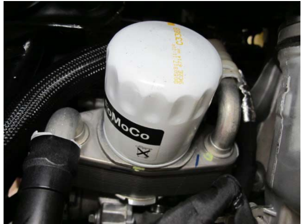
Fig. 1-d: Remove Oil Filter
