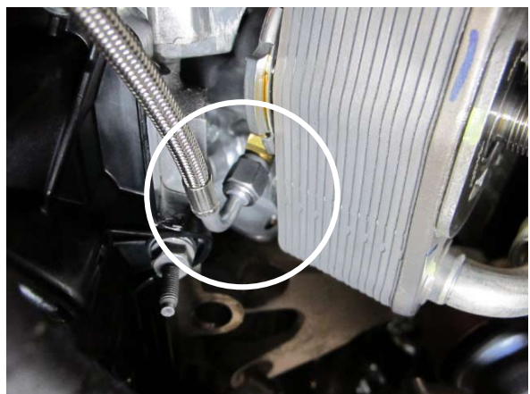
Fig. 1-r: Position 1/8" NPT 45° x -4 JIC Fitting And Install Steel Braided Oil Feed Line
