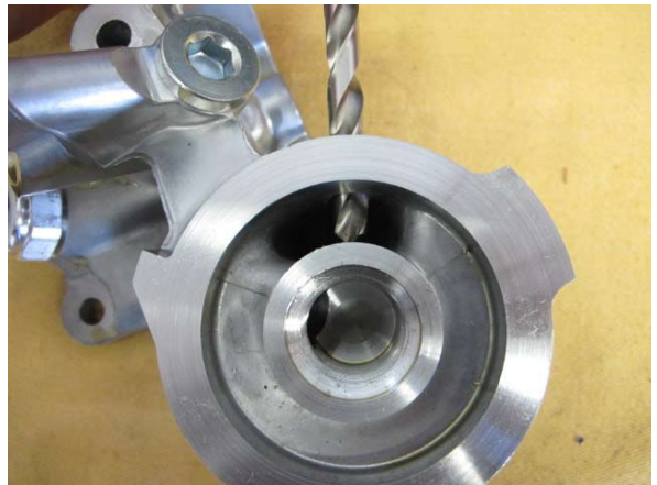
Fig. 1-n: Verify Hole Location
