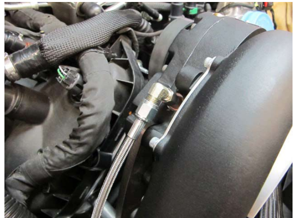
Fig. 1-w: Install Steel Braided Oil Feed Line
