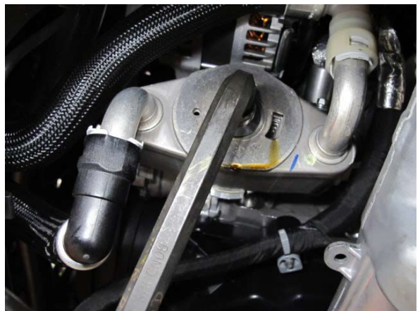
Fig. 1-f: Remove Threaded Oil Tube
