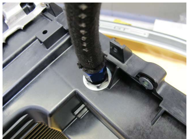
Fig. 2-f: Secure Oil Drain Line
