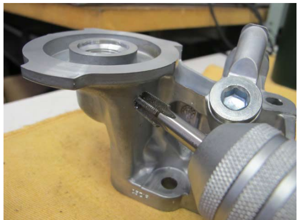
Fig. 1-o: Tap Hole Using 1/8" NPT Tap
