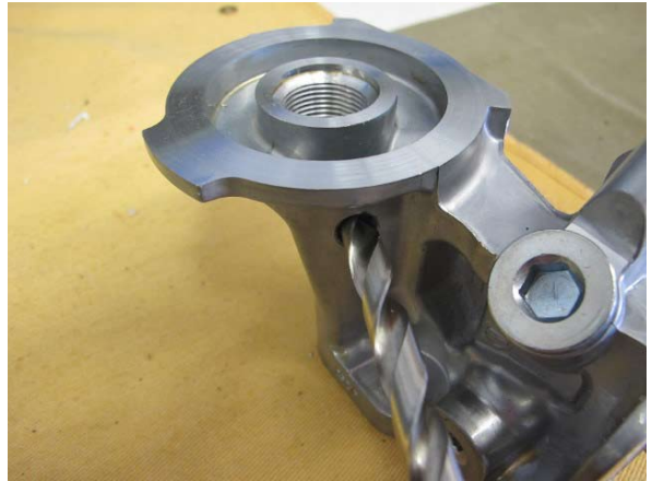
Fig. 1-m: Drill Through Center Punch
