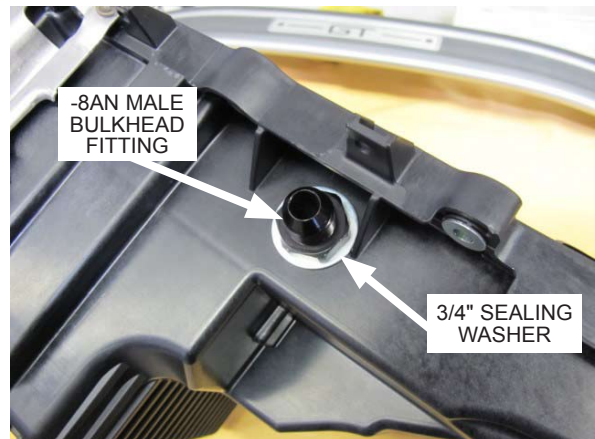
Fig. 2-d: Install -8AN Bulkhead Fitting
