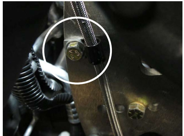
Fig. 1-t: Route Steel Braided Oil Feed Line Through Adel Clamp
