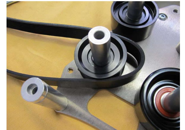
Fig. 2-b: Install 8-Rib serpentine belt as shown.
