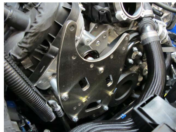
Fig. 2-f: Install 8-Rib drive supercharger mounting bracket assembly.
