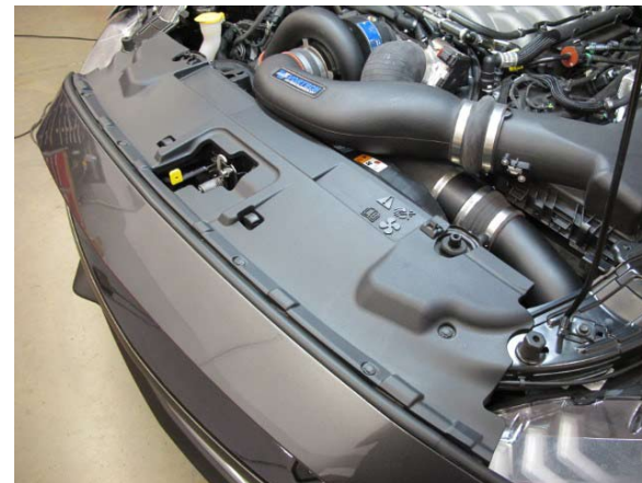
Fig. 1-d: Remove radiator support cover.
