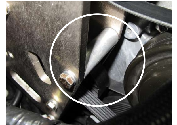
Fig. 3-h: Reinstall these spacers and hardware.
