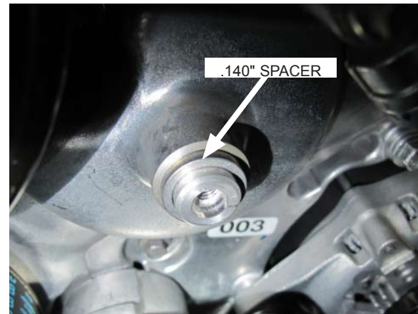
Fig. 2-j: Install .140" spacer onto pilot.
