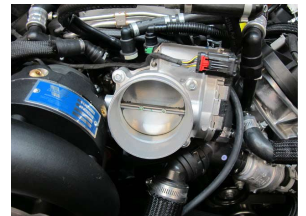
Fig. 1-o: Remove throttle body.
