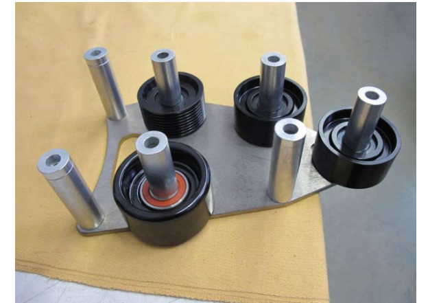
Fig. 2-a: Assemble 8-Rib supercharger mounting bracket assembly.
