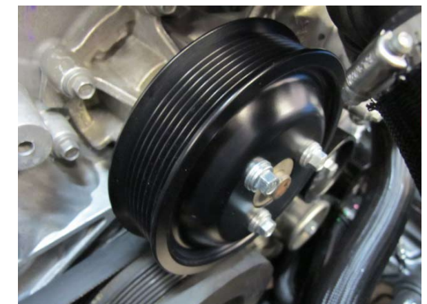
Fig. 2-o: Install 8-rib water pump pulley.
