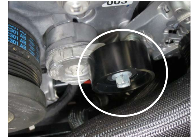
Fig. 2-n: Install offset smooth idler pulley and secure using OEM screw only.
