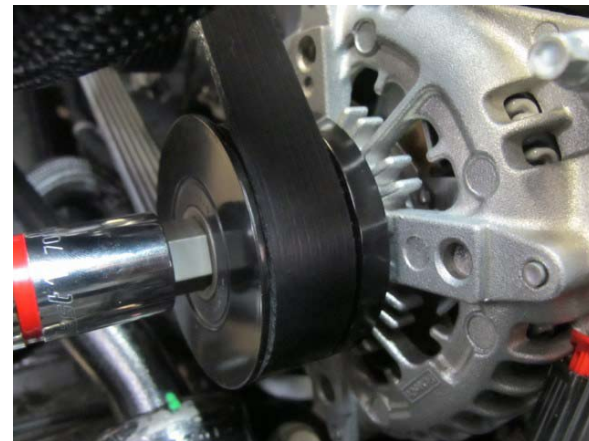
Fig. 2-p: Remove 6-rib alternator pulley.
