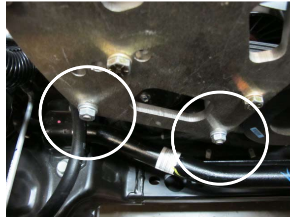
Fig. 1-v: Remove 2x nuts and/or 2x M8 x 200mm threaded studs.
