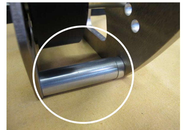
Fig. 2-c: 2x 2.730" spacers and 2x .280" spacers.
