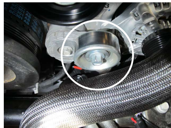
Fig. 2-l: Remove OEM smooth idler pulley located on belt tensioner.
