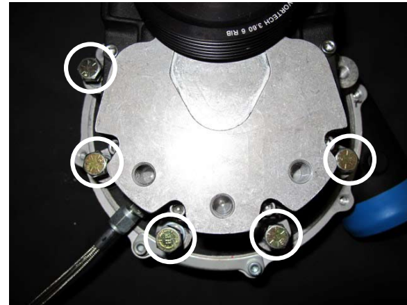
Fig. 3-d: Lubricate supercharger mounting boss threads.
