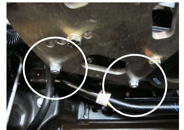
Fig. 2-i: Install 2x M8 nuts and 2x 5/16" washers.
