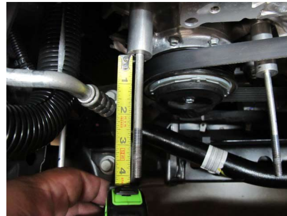
Fig. 2-e: Install 1x 2.058" and 1x 2.146" spacers.
