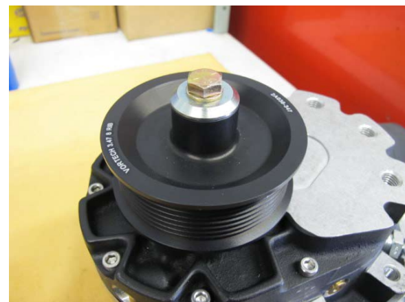
Fig. 2-r: Install 8-rib supercharger pulley.
