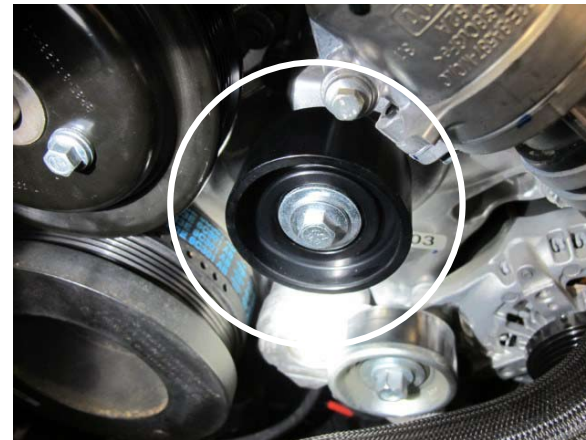
Fig. 2-k: Install smooth idler pulley and secure using OEM screw and washer.
