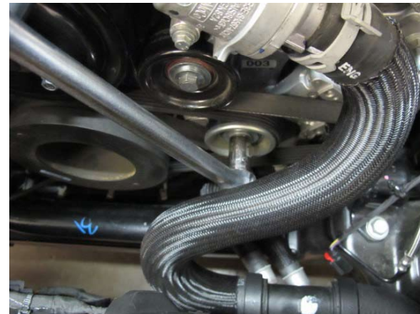
Fig. 1-k: Remove serpentine drive belt.
