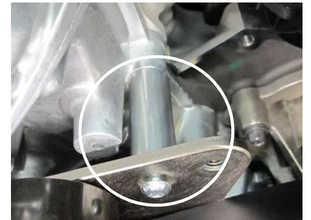
Fig. 2-g: Install 1x 2.058" spacer.
