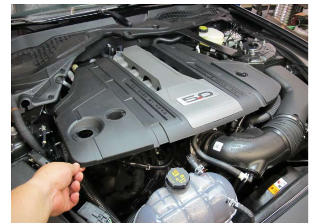
Fig. 1-c: Remove engine cover.
