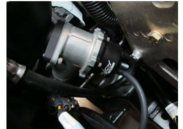
Fig. 1-n: Disconnect vacuum line from bypass valve.
