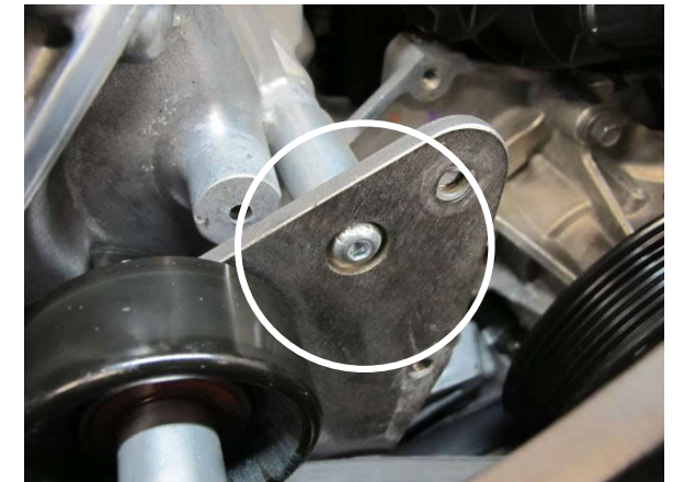
Fig. 1-t: Remove button head screw from passenger side of engine.
