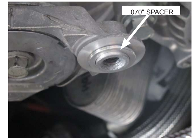
Fig. 2-m: Install .070" spacer onto pilot.
