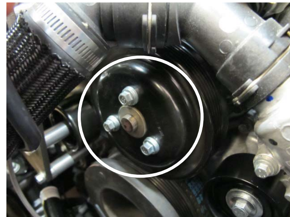
Fig. 1-j: Loosen water pump pulley screws.
