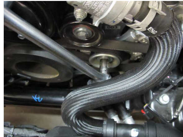
Fig. 3-j: Install supercharger drive belt.
