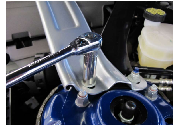
Fig. 1-b: Remove strut tower brace.
