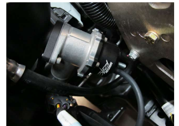
Fig. 3-i: Reconnect vacuum line to bypass valve.
