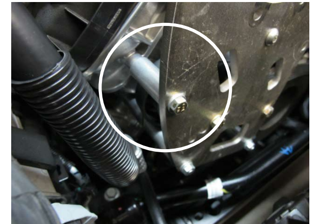
Fig. 2-h: Install 1x 1.928" and 1x .280" spacers.
