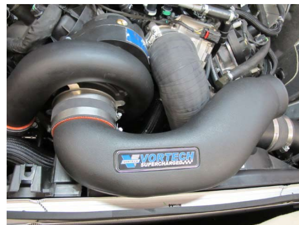
Fig. 1-f: Remove air inlet tube.
