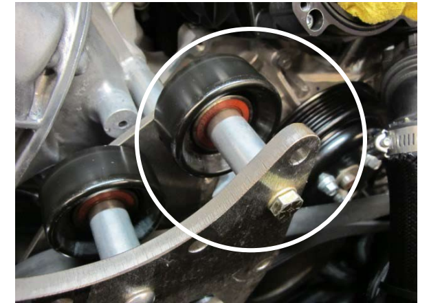
Fig. 1-s: Remove upper smooth idler pulley.
