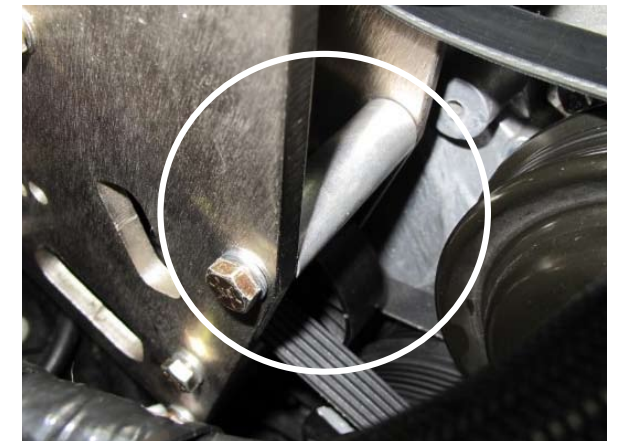
Fig. 3-a: Temporarily remove these spacers and hardware.
